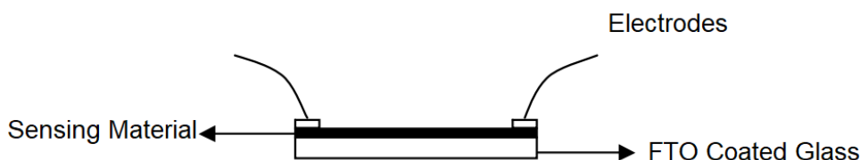
Figure 4. 16 Schematic representation of sensor fabricated
